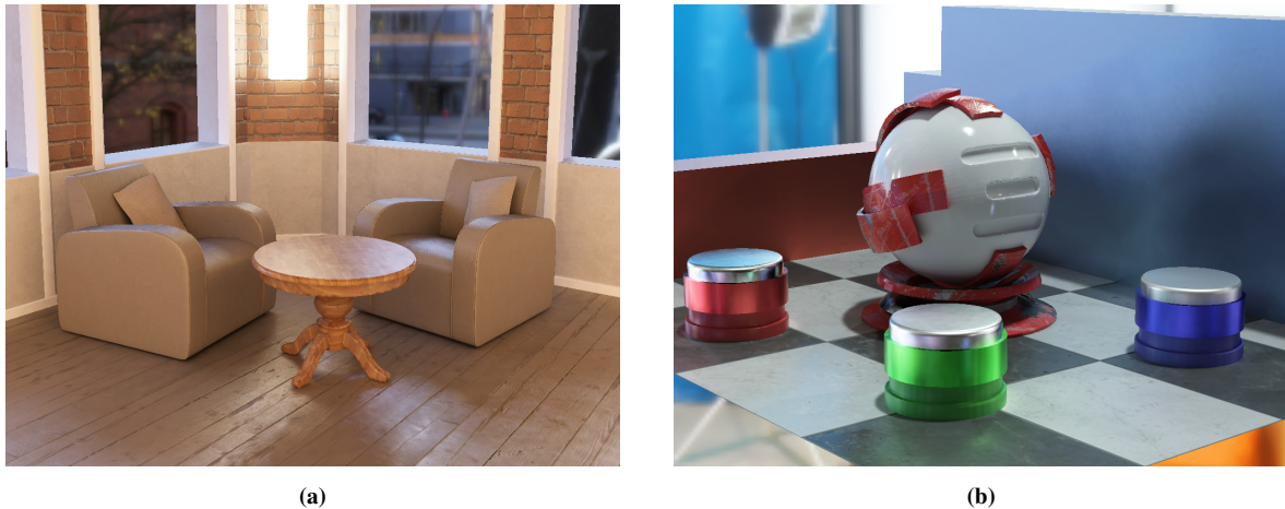
Figure 1: Two scenes rendered with our method. The local light field for any fragment is available as a precomputed set of 16 Spherical Gaussians in a light-field texture ( 512 \times 512 , 56MB). A similar texture contains the attenuation factor for a preconvolved environment map. The combined result is images with full global illumination for glossy surfaces rendered in just over a millisecond at 1080p resolution.
