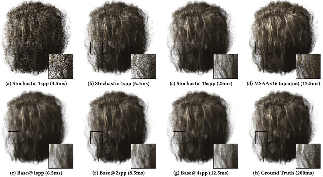
Figure 5: Result of rendering the hair using different methods: (a), (b), and (c) use stochastic transparency at different SPP; (d) is the hair rendered with MSAAx16 without transparency; (e), (f), and (g) are the results of our network for different SPP; (h) is the super-sampled reference image. In parentheses is the total time to render a frame.
